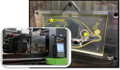
Structural electronics product by injection over-molding
